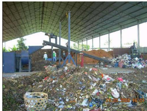
New composting facility designed for capacity to handle waste about 100 ton/day
